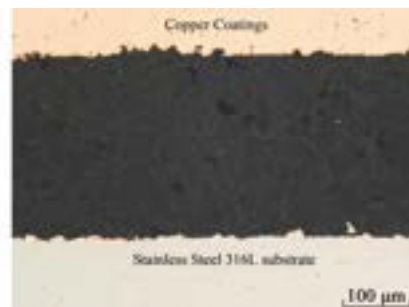
Fig. 15. Cross-sections of fractured Cu coatings on SS 316 L substrates.
