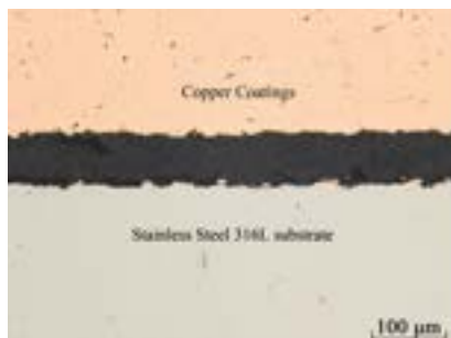
Fig. 15. Cross-sections of fractured Cu coatings on SS 316 L substrates.
