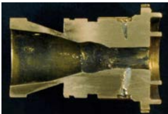
(b) Severe erosion for a relatively long time usage
